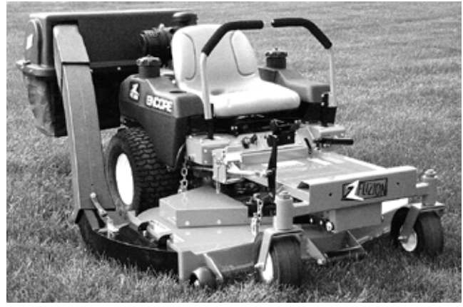
Figure 10 This completes the installation of your new Encore grass catcher system. Note that when engaging the PTO switch; always make certain the unit is running 3/4 to full throttle so as to prevent stalling.
