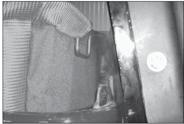
Figure 4 Install the grass bags by sliding the mounting hook into the hanger mount.
