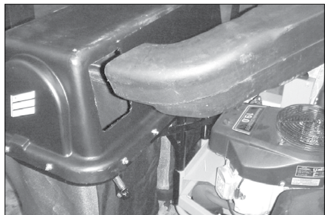
Figure 6 Slide the upper grass tube into the opening of the catcher hood.
