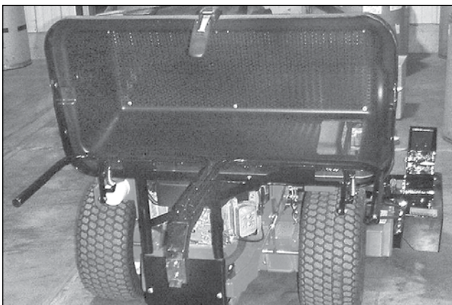
Figure 3 Slide the assembled hood and frame onto the rear skid bars. Let the assembly slide all the way down to the grass catcher brace.
